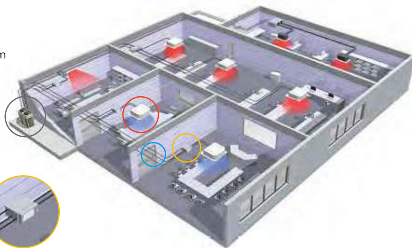
Single and multi Branch Selector boxes: allows the individual switching of indoor units between heating and cooling
